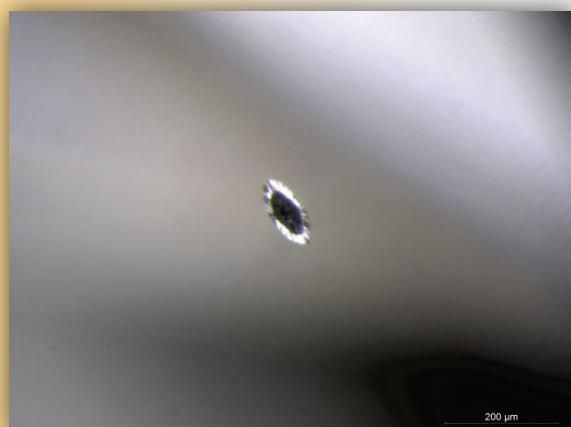
Fig. 2: Inclusion modified by the HPHT treatment (discoid fracture), stone N° 2, dark field illumination. © GGTL Laboratories - 2013
